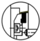
Multiple arrangement metal hard sealed structure
